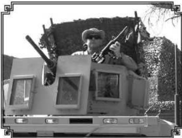
Pictured is an up-armored HMMWV, referred to as a gun truck. Lt. Col. Smith is in the turret with a .50 caliber crew-served weapon and a M-4 assault rifle. The gun-truck is effective against many improvised explosive devices and resistant to small arms fire.
